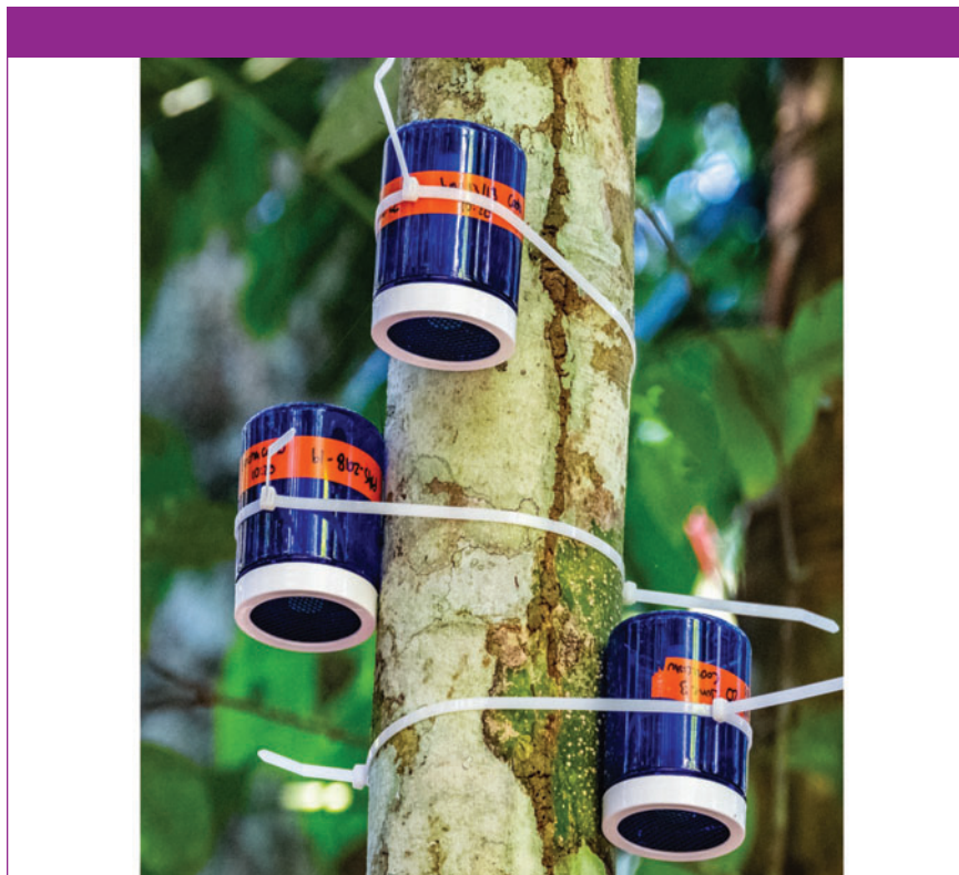
Figure 11: CINCIA's passive mercury samplers can be attached to any vertical support including street lamps, power poles, or trees (Photo credit: CINCIA).
