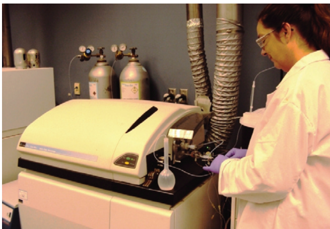
PerkinElmer ELAN DRC-e ICP-MS in Nutra's QA/QC laboratory.
