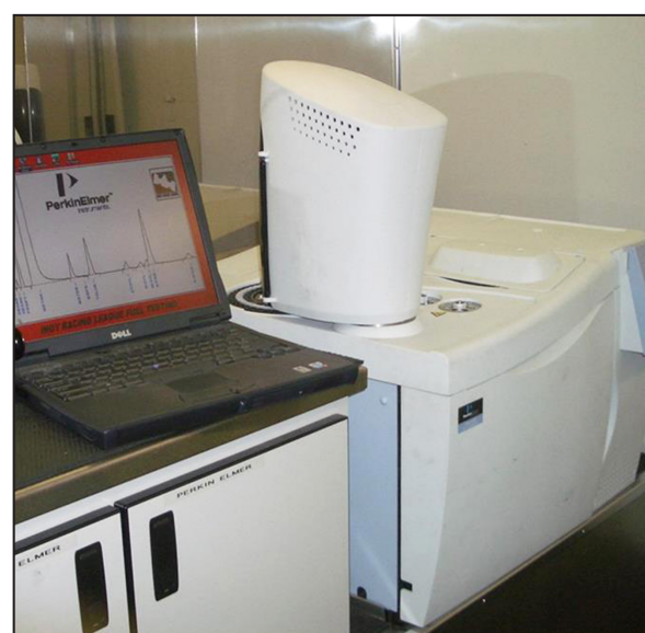
Figure 4: PerkinElmer's Clarus GC System used to test IndyCar fuel (Courtesy of PerkinElmer Inc.)
