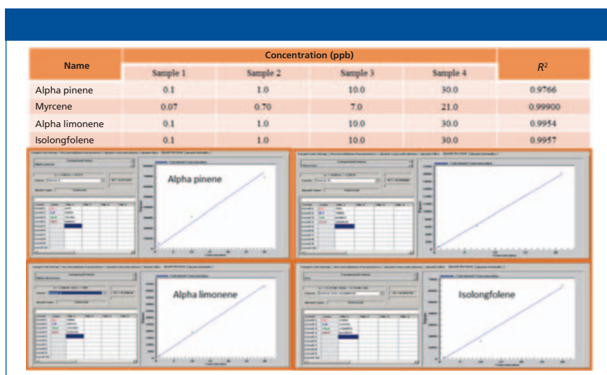
Figure 3: Calibration plots of the four terpene compounds.
